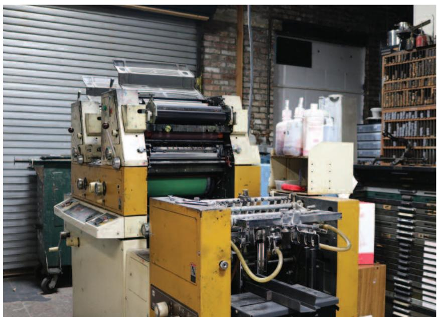
An offset press; a quick and efficient machine for printing book interiors
